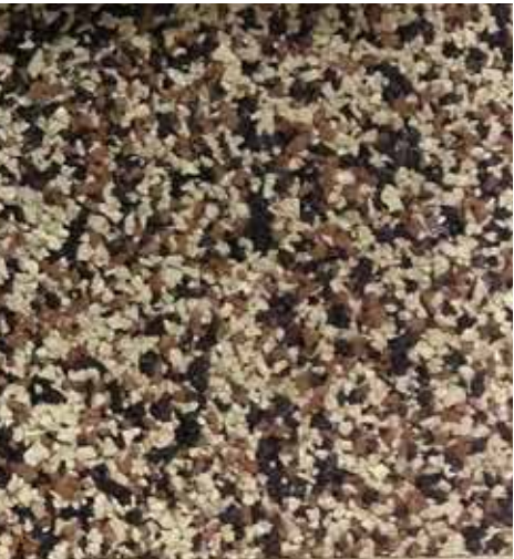
1. Safety surfacing: Resin bound rubber crumb, colour mix specified for play mound play, black 25%, beige 25%, brown 25%, eggshell 25%, colour mix for other areas TBC
